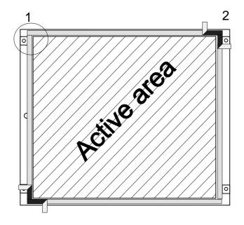
1. Install double sided tapes to metal frame. If you want "dustproof" installation, make sure that the tape ends are fitted well.
