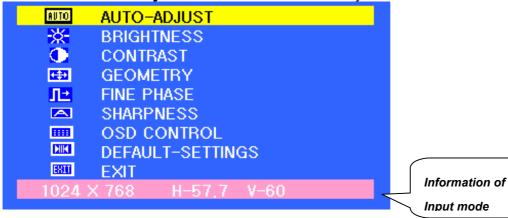
AUTO-ADJUST: Adjust position, horizontal size, and phase automatically
